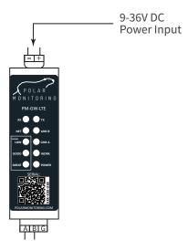
In cases where the PM Gateway is getting power from the device it is monitoring the 0V pins are already connected.
