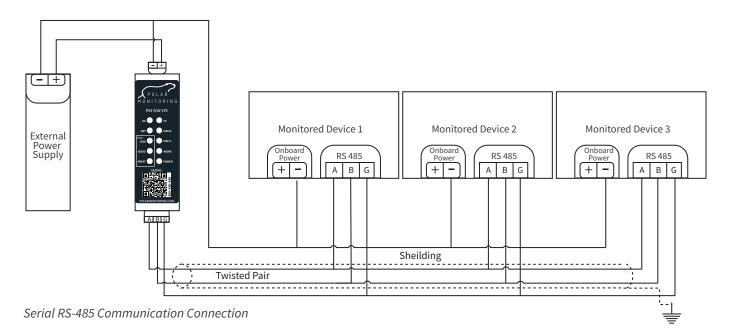
The communication port is for RS-485 connection only. It will connect the device to be monitored to the PM Gateway and therefore to the cloud. Care must be taken to connect this correctly as improper wiring can compromise the data collection procedure.
