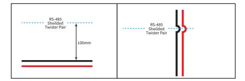
Communications cables should be kept at least 100mm distance from any high-power cables.
