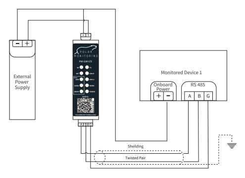
When the PM Gateway is monitoring multiple devices on a single Gateway then each of the 0V DC points on the devices must be wired together to avoid ground loops on the system.
